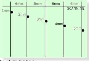
Figure 1 - Near Field Target Wire Diameter 0.1 mm
