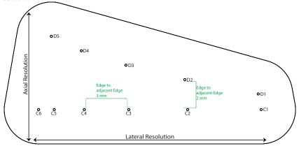
Figure 4 - Combined Axial/Lateral Resolution Target at 10.5 cm depth
